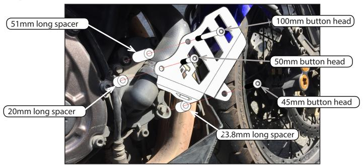
Follow the exploded view in the image to assemble the guard to the water pump housing. Use a 4mm allen tool to tighten each of the button head fasteners. Tighten all (3) M6 bolts to 8.7nm
