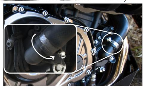
Perform this installation with the engine cold. Start by laying your Tenere on its left side. Use a phillips head screw driver to loosen the pipe clamp fastener until you can remove the clamp. Flip the pipe clamp around and re-install it. Tighten the pipe clamp back down.
