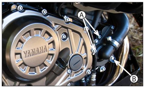
(A) Use a 5mm allen tool to remove the two indicated OEM fasteners, then (B) use an 8mm socket to remove the hex fastener indicated. You will not reuse these fasteners.
